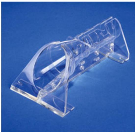
Easy to use mouse and rat restrainer specifically designed for tail vein injections
