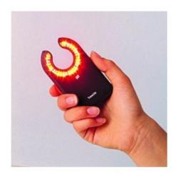
the simplest device to illuminates mouse tail for easy injection or sampling
