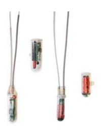
telemetry implants for rodents allowing measurements of temperature, activity and heart rate
