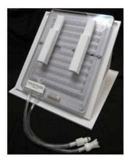
Heated pad to be installed on a tiltable work stand
