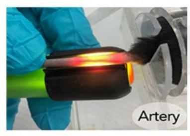
the simplest device to illuminates mouse tail for easy injection or sampling
