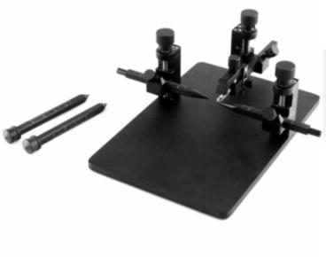
To be mounted on a stereotaxic frame - Delivered with 20° and 45° ear bars
