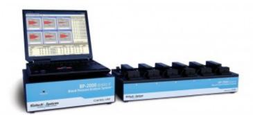
The world's leading non-invasive blood pressure analyzer for mice and rats: a state-of-the-art, expandable instrument based on transmission photoplethysmography, highly accurate and reliable for measurements on animals ranging from small mice to extremely large rats. Comes with a powerful, yet intuitive, dedicated software to review and verify your data, and export your results.
