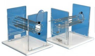
Restrainer usable on a variety of animals on a diverse weight range and providing easy access of the entire body - Especially used for obesity studies
