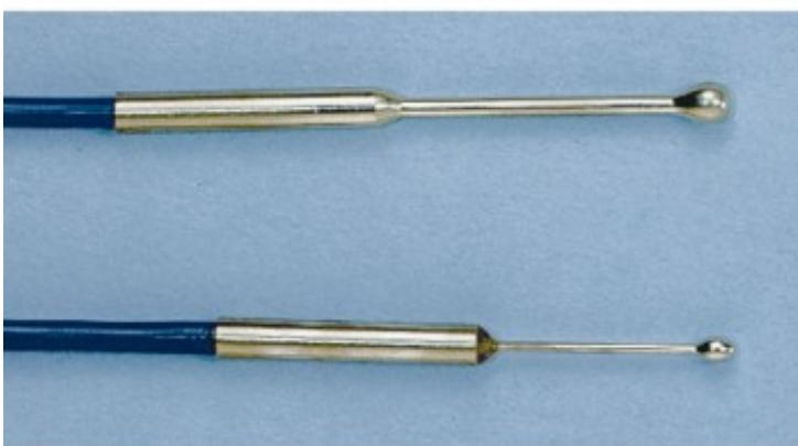
Stainless steel rectal probes for the measure of core temperature on conscious or anaesthetized animals
