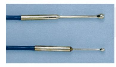
Stainless steel rectal probes for the measure of core temperature on conscious or anaesthetized animals
