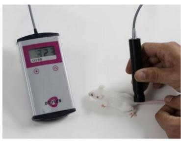
Very fast and contactless, infrared temperature measurement for small rodents (mouse and rat) - specially design to allow measurements on small surface, like the tail of a mouse, with high accuracy and repeatability.
